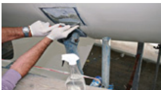
Wet scrape to remove old antifouling
