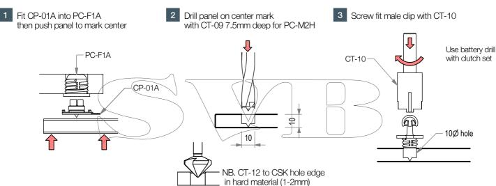
INSTALLING ADHESIVE FIT MALE CLIPS (first complete steps 1 to 3, page 1)
