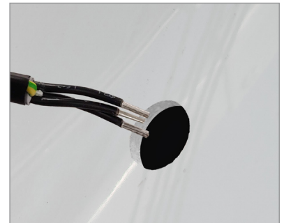
[Figure 14] Insert the generator cable into the hole so that the connector remains outside of the boat
