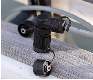
[Figure 4 ] Feedthrough connectors installed in the boat
