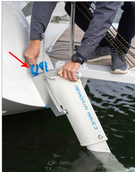
[Figure 28] Lock the outboard unit onto the rail by pushing the handle down to the bottom position
