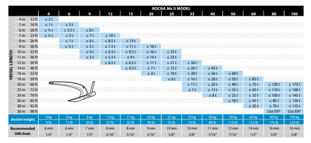
**OUR SIZING IS CONSERVATIVE**: Our sizing recommendations are intended to provide an anchor adequate for use in most conditions. We base our calculations on 50 knots of wind, associated surge, and poor holding bottoms. Recommendations are incomparable with other anchor producers.
