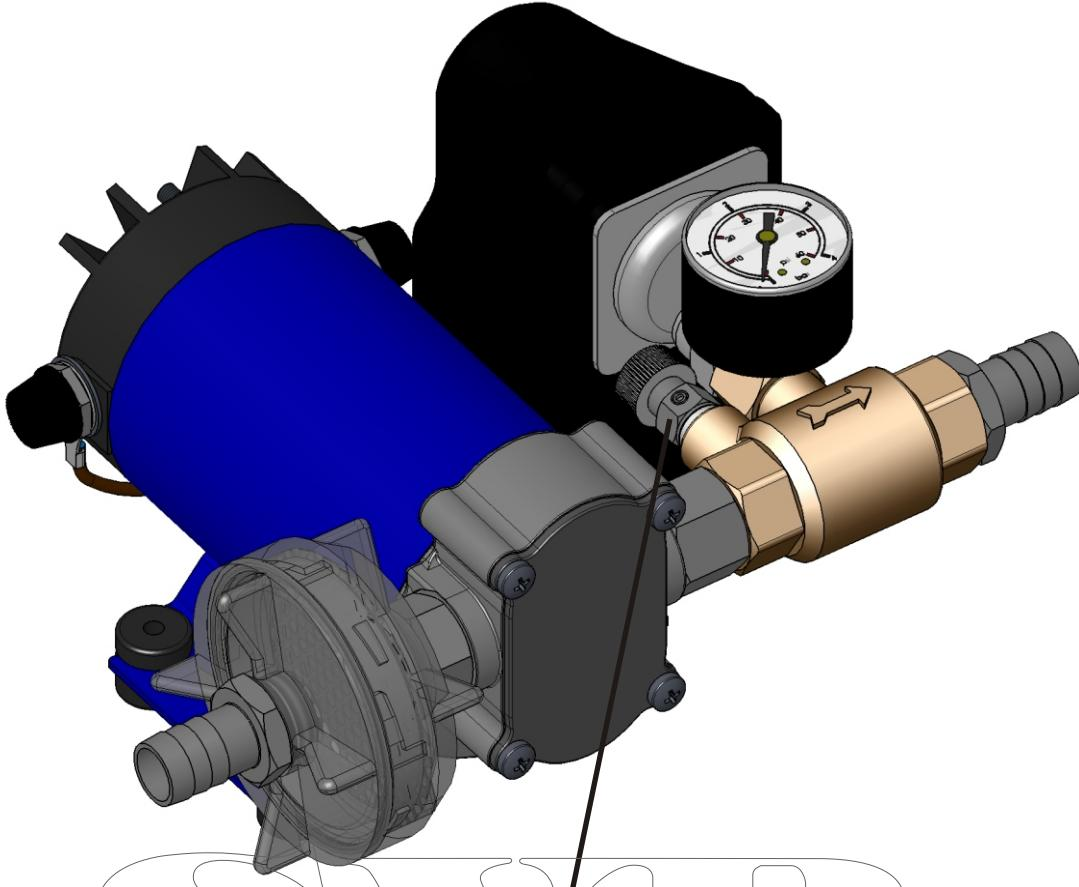
When starting the pump slightly open the small valve located next to the pressure switch, in order to let the air out and facilitate the pump priming. As soon as the pump is operating close the small valve.
