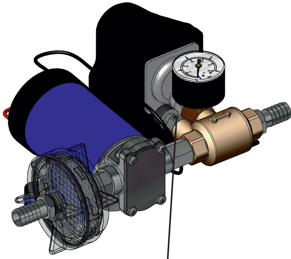
When starting the pump slightly open the small valve located next to the pressure switch, in order to let the air out and facilitate the pump priming. As soon as the pump is operating close the small valve.
