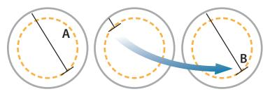
When true motion is selected, the true motion reset option is available from the menu. This allows for manually resetting the radar image and vessel symbol to its starting position.
