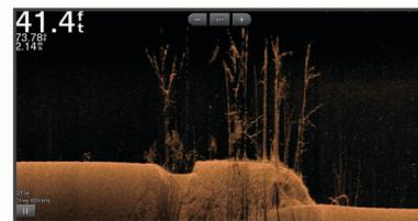
Traditional transducers emit a conical beam. The Garmin ClearVü scanning sonar technology emits two narrow beams, similar to the shape of the beam in a copying machine. These beams provide a clearer, picture-like image of what is beneath the boat.
