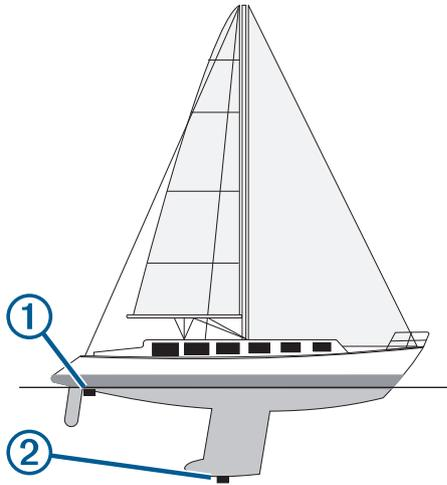
2 Select **Settings > My Vessel > Depth and Anchoring > Keel Offset**.
