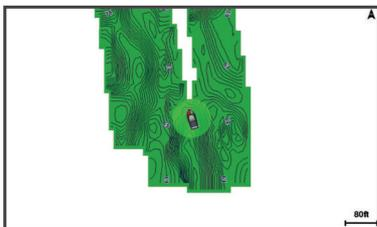
A green circle indicates good depth and GPS position, and a speed under 16 km/h (10 mph). A yellow circle indicates good
