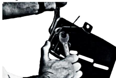
4. Tighten the bolt with a wrench and lock it by firmly tightening the shallow lock-nut to be put on the end of the bolt (see arrow).
