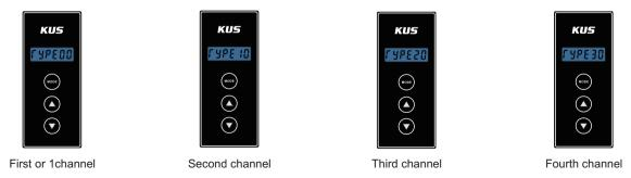
Notes: 1. For four channel adapter, short press MODE to switch the channel what need to set.
