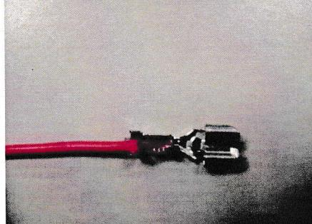
A photograph showing the stripped end of a single wire being inserted into a crimp terminal or connector housing.                                                                                                         | <ul style="list-style-type: none"><li>• Plaats het uiteinde van de kabel in de kabelschoen.</li></ul> |
