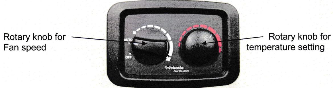
The rotary knob has 7 settings for the fan speed: Off, Automatic and five settings for manual control of the fan. The knob for temperature setting is variable. The indicators of both knobs light up in red.
