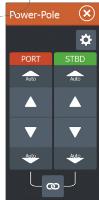
Dual Power-Poles controller
