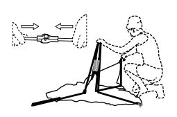
2. With central hub upright, unfold the poles and lock the joint.
