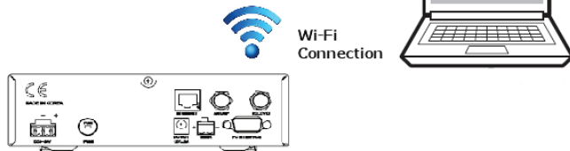
Figure 27 : ACU to PC Wifi Connection
