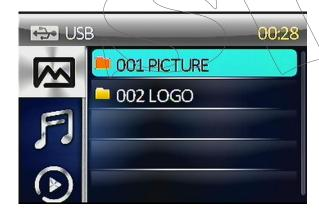
Press the direction buttons to select your desired FOLDER, then press the ENT or button to open the FOLDER, or play the selected file. When displaying the root menu, you can also use the number buttons to select the serial number of the file and play the file.
