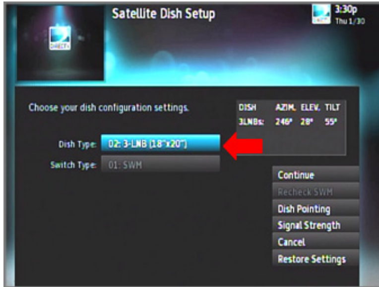
Figure 5-6 Satellite Dish Setup on DIRECTV Receiver
