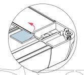
Turn over and remove protective covers from adhesive pads in each corner.
