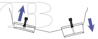
The starboard button controls the starboard tab upwards first and then the port tab downwards.
