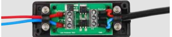
With this hookup, the cells are protected with 2 bypass diodes against the hot spot effect.
