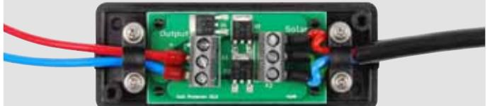
With this hookup, the cells are protected with 2 bypass diodes against the hot spot effect and the additional blocking diode protects against reverse current back into the module. By damage to a module or cable by several modules in parallel operation, an influence can be prevented on the other modules with the use of the blocking diode.
