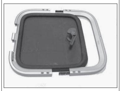
1.7) The seal is stretched over the Acrylic but may have been glued in place to aid assembly. If the seal is removed from the acrylic the acrylic will need cleaning, solvents should not be used
