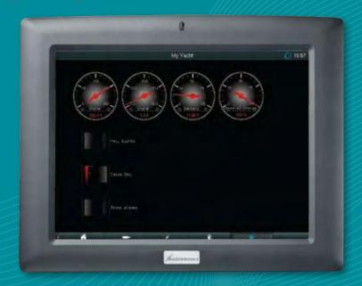
**Power Flow screen:** Graphical system layout with visualization of voltages and animation of currents. Incorrect line voltages are shown in red, inactive circuits in grey and activated circuits in a designated colour.
