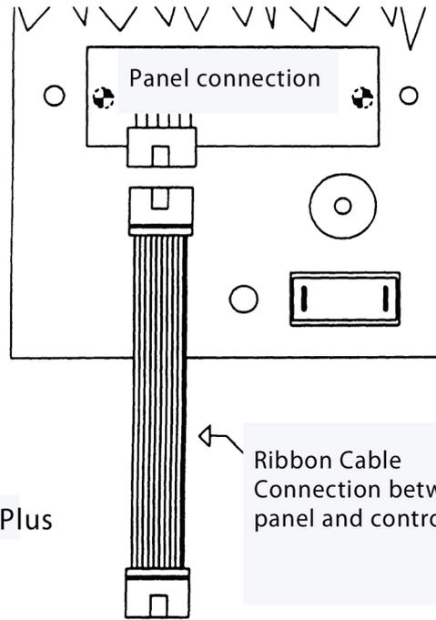
Ribbon Cable Connection between panel and control box
