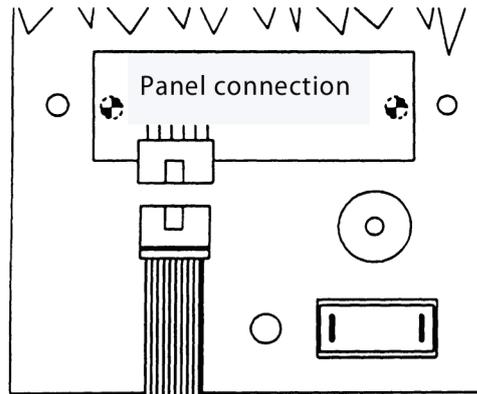
Ribbon Cable Connection between panel and control box
