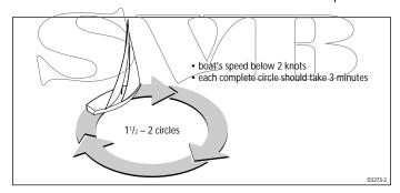
4. Keep turning your boat until the display changes to show the amount of deviation the autopilot has detected (this should take between 1<sup>1</sup>/<sub>2</sub> t o2 complete circles). The deviation alternates with the autopilot's current heading every second.
