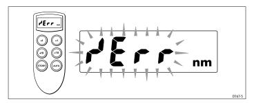
The tiller pilot displays this message if you select Track mode when the navigator has lost its fix. This display will clear as soon as the navigator regains its fix.
