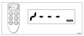
This error message indicates that data has not been received. The most likely reason is a cabling error – either open circuit, short circuit or wires reversed.
