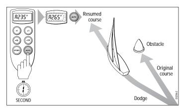
**Note:** If you do not pressauto while the display is flashing, the autopilot will maintain the current heading.
