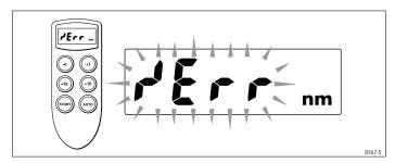
The tiller pilot displays this message if you select Track mode when the autopilot is not receiving any navigation data.
