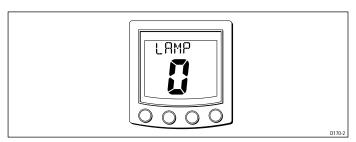
3. The tiller pilot should immediately respond by switching off its display illumination. If the illumination does not switch off, there is a cabling fault between the tiller pilot and the instruments or control unit.
