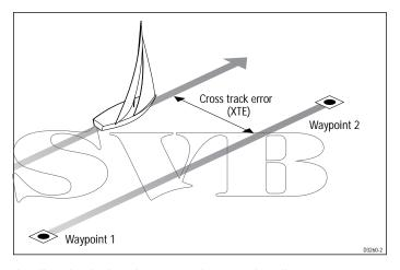
The tiller pilot displays the cross track error in the following ways:
