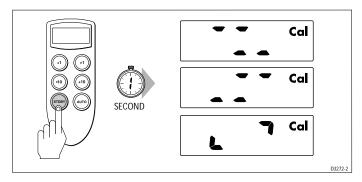
3. Keeping boat speed below 2 knots, use the **-10** and **+10** keys to turn the boat in slow circles. You should take at least 3 minutes to complete each 360°.
