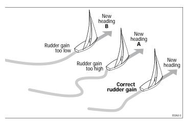
**Note:** It is easier to recognize these actions in calm sea conditions where wave action does not mask basic steering performance.
