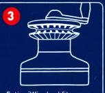
Entire 'Wincher' fits over winch – ribs face downwards & flange sits on winch lip.
