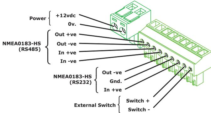
Figure 2.1 - Connector wiring
