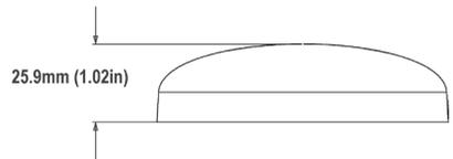
Figure 5.2 - Navico GPS 1330-N Antenna dimensions
