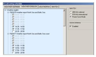
Messages which mutually overlap are locked in the broadcasting schedule. Thus it is ensured that all selected messages can be received. A manual choice of the reception frequency is not necessary. The WIBE searchs automatically for the best reception signal before recording a message.
