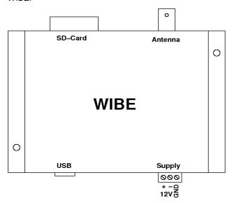
The antenna socket (BNC) can be connected with an active antenna (12V) or a passive antenna (e.g. isolated backstay with passiv balun). In the WIBE software you have to determine which antenna is connected. This setting can be done either via icon or via menu Settings -> Broadcasting schedule:
