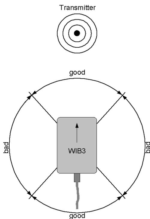
The internal ferrite rod antenna of the WIB3 has a directionality. For good reception the equipment must be operating flat lying. With small distance to the transmitter the directionality of the antenna will become hardly noticeable. The range of the bad receipt (see illustration) is hardly to be determined.
