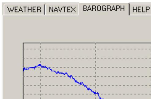
The third tab contains the BAROGRAPH. The measuring data are represented in the diagram from left to right. I.e. the current measured value is on the right side of the curve. The barograph has a measuring interval of one minute and resolution of 0,1hPa.
