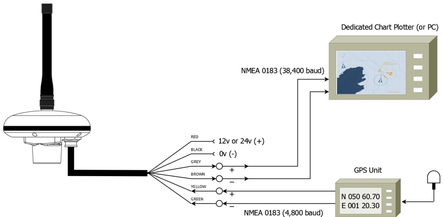
**NOTE:** Connection of the GPS Unit to the ANT200 is not mandatory but can be useful in some installations where the dedicated chart plotter only has one NMEA Input port
