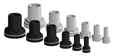
The Skin Fitting body and nut are moulded from glass fibre reinforced nylon composite. High strength, high-modulus glass fibres impregnated into the nylon provide dramatic strength, stiffness, toughness and dimensional stability. These properties allow a significant weight reduction over metallic fittings.
